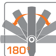
180° flex head has 13 Locking Positions.
